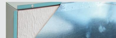
PF Board is high function, fire-resistant insulation material with the energy efficiency maximized by foaming thermosetting polymer with eco-friendly foaming gas(non-freon gas). With fine particles sized only 1/10 of Styrofoam, PF Board has thin but rigid internal structure that will keep up the insulation performance for over 25 years.
